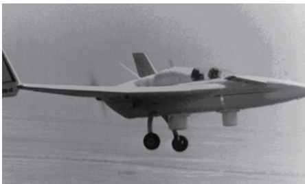
Figure 1: CM-30 carrying Medfli/MASS equipment
